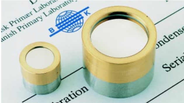
Fig. 1. The Brüel & Kjær Laboratory Standard Microphones Type 4160 (23.77 mm diameter – named one inch) and Type 4180 (half inch diameter) are the Reference Standard Microphones which are most commonly used by national and other well established calibration laboratories. The microphones meet the requirements valid for types LS2p and LS1p of the international standard IEC 61094-1
